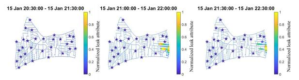
Figure 3 Leak localization results up to 23:00 hrs on 15th of January, 2019
