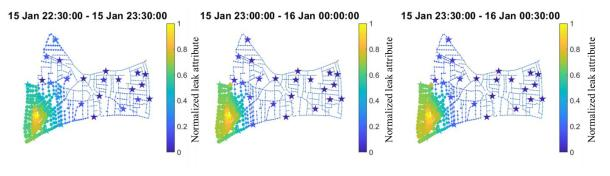
Figure 4 Leak localization results before, during and after 23:00 hrs on 15th of January, 2019
