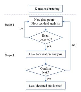
Figure 1 Leak detection and localization process
