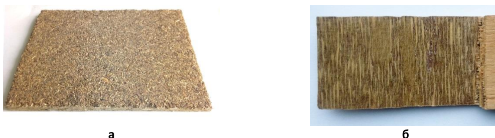
Figure 1: Photos of the samples of the adhesive (alkaline aluminosilicate binder)-bonded wood-based materials (a) – particle boards and (b) – plywood after testing for internal bond
