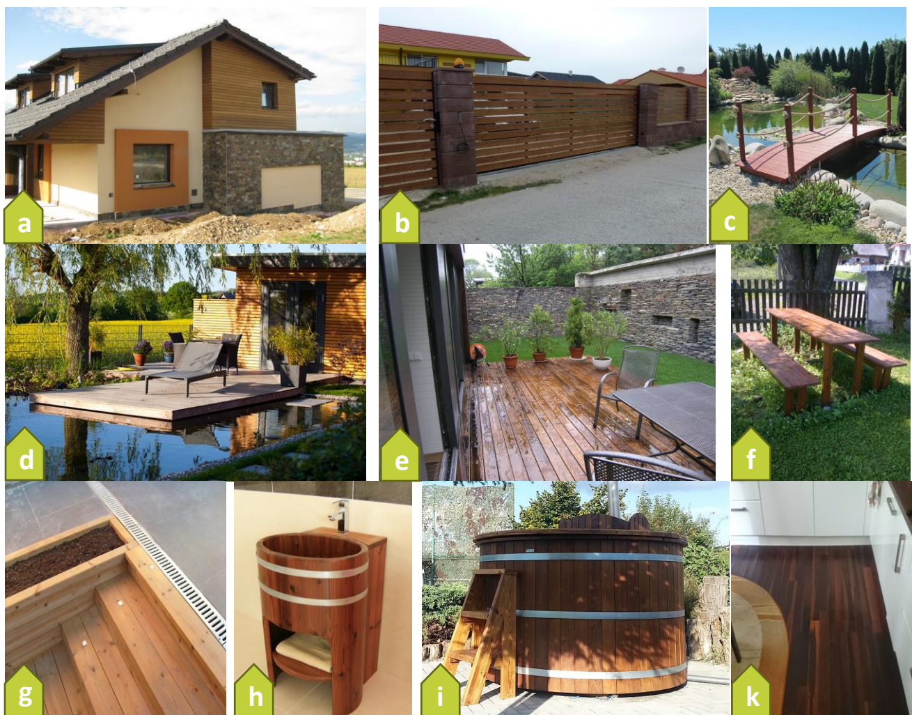
Figure 1: Thermally modified pine wood facade (a), gate and fence (b), bridge (c), terrace by the pool (d), garden furniture (f), flowerpots and stairs (g), washbasin (h). Thermally modified ash or beech wood terrace (e), bathing or cooling off tub (i). Thermally modified quercus parquet floors (k). (Foto: references from companies RM drevo s.r.o., TECHNI-PAL and Rostaco Slovakia s.r.o.)
