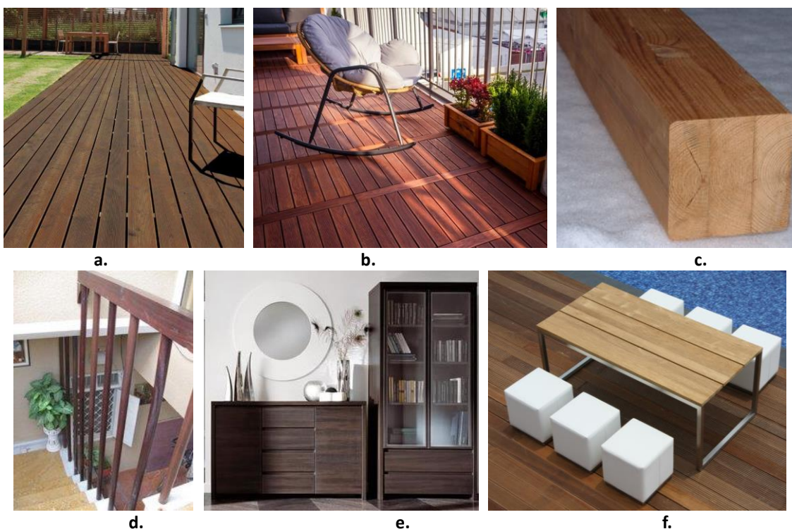
Figure 1. Thermally modified pine for decking (image provided from http://www.pardoseli-lemn.ro/deck/autohton/pin-termotratat/ ), thermally modified ash for decking and flooring (image provided from https://decolandia.ro/terase-din-lemn-si-pardoseli-exterioare/podele-terasa-decking--frasin-thermo ), reinforced beams made from thermally treated pine (image provided from http://www.lemntratat.ro/detaliiprodus/amenajari_lemn_terase/grinzi_stratificate_neportante_molid_termotratat/grinzi_stratificate_5/16/18.html ), balusters of thermally treated ash (image provided from www.lemntratat.ro/detaliiprodus/dusumele_si_lambriuri/balustri_si_mana_curenta_lemn_termotratat/balustrii_si_mana_curenta/7/38/34.html ), furniture from massive thermal treated hardwoods – beech, oak or ash (image provided from www.lemntratat.ro/detaliiprodus/dusumele_si_lambriuri/mobilier_interior_lemn_termotratat_masiv/mobilier/7/41/36.html ), outdoor table (image provided from www.lemntratat.ro/categorii/amenajari_lemn_terase/5.html )
