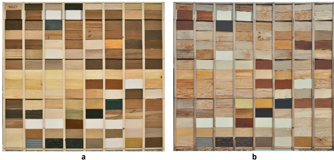
Figure 1: Appearance of investigated samples at the beginning of the test (a) and after 12 months of natural weathering at the southern exposure (b).
