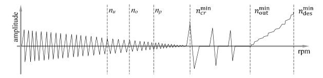
Fig. 1. Characteristic rotational speeds of the circular saw blade according to Stakhiev [17]:  $n_u$  – universal;  $n_o$  – optimal;  $n_p$  – permissible;  $n_{cr}^{\min}$  – the lowest critical;  $n_{out}^{\min}$  – the lowest self-excited;  $n_{des}^{\min}$  – destructive
