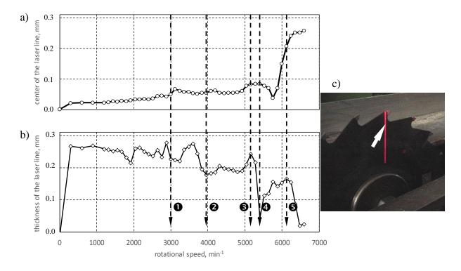
Fig. 7. Change of the saw deviation (a) and axial run-out (b) of the saw blade in the zone close to the gullet (c) versus the spindle rotational speeds;  $\mathbf{0}$  - typical,  $\mathbf{2}$  - first optimal,  $\mathbf{3}$  - first critical,  $\mathbf{4}$  - second optimal,  $\mathbf{5}$  - second critical
