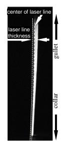
Fig. 4. Processing of the laser line image
