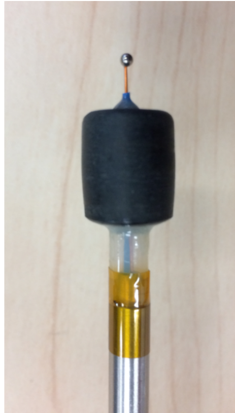
"new sensor" Rod + umbrella (bakelite) + ball
