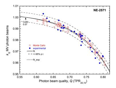
Figure 1: Values of  $k_Q$  for megavoltage photon beams obtained from Monte Carlo calculations by different research groups (open circles) and measured at standards laboratories (filled circles) for a NE-2571 Farmer-type ionization chamber. The solid line is a fit to the total of 154 data points using Eq. (6) and the dashed lines are the 95% prediction limits of the fit. The short-dashed line corresponds to the fit of the 28 experimental data points.
