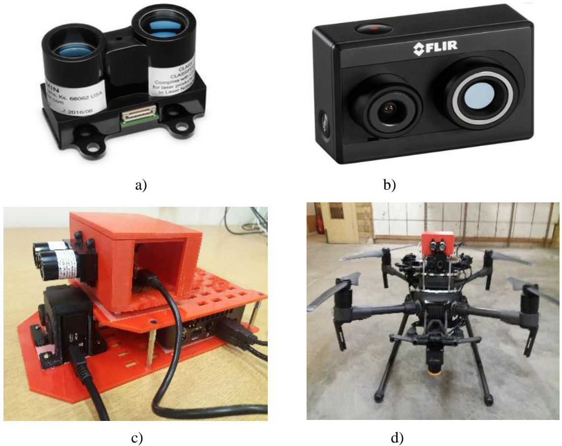
Fig. 2. Software and hardware system: a) LIDAR laser; b) FLIR Duo R; c) Connecting LIDAR and FLIR Duo R to the Intel® NUC8; d) DJI MATRICE M210 V2 drone with sensors installed on it.
