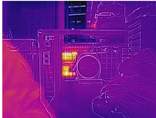
Fig.7. Real time temperature data extraction from thermal images: a) visual image; b) thermal image in .tiff format; c) extracted Celsius degrees temperatures and saved in a .jpeg file; d) applying a colormap in OpenCV on c) image; e) MSX enhanced radiometric jpeg thermal image as taken by the Flir Duo R dual-sensor thermal camera.
