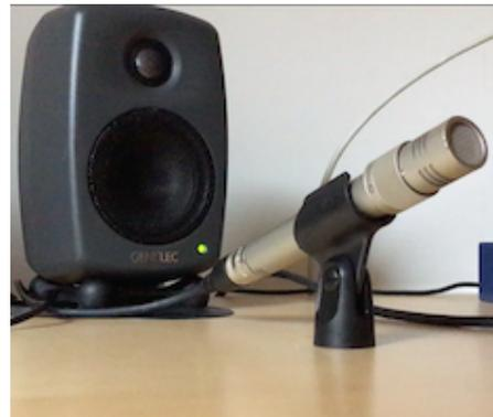
Figure 2. A minimal auralization system consisting of one microphone and speaker. Note that this system would be prone to feedback at frequencies associated with the direct path and first reflection (off the table).
