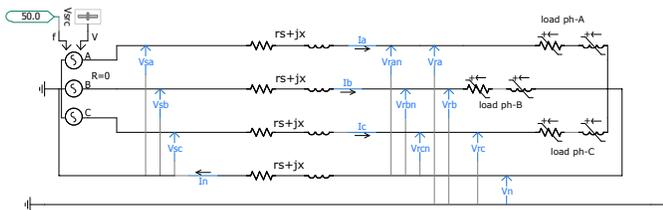
Fig. 4. Lab cable and measurement set-up.
