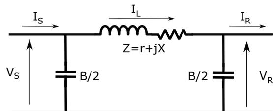
Fig. 1. Nominal Pi model for a medium length medium voltage line
