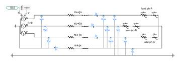
Fig. 4. Lab cable and measurement set-up.
