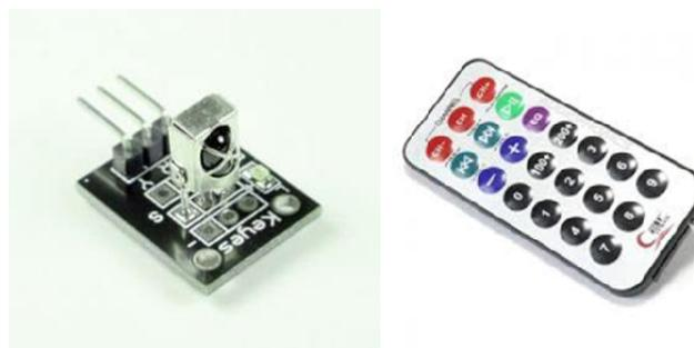
Fig. 6 IR Receiver and Transmitter
