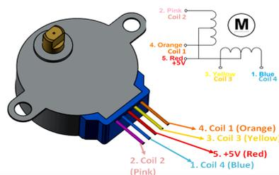
Fig. 2 Pinout Diagram of Stepper Motor
