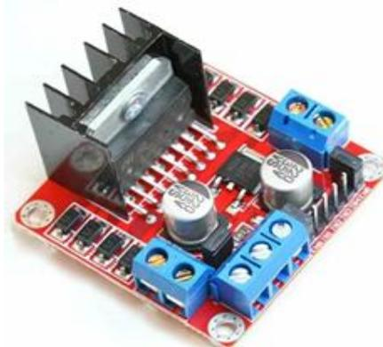
Fig.10 ULN 2003 Board Fig.11 L298N Motor Driver
