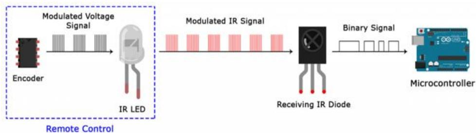
Fig.7 IR Signal Modulation
