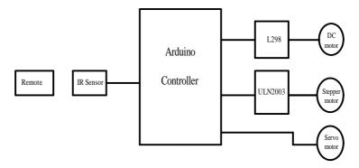
Fig. 4 Block Diagram of System
