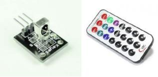
Fig. 6 IR Receiver and Transmitter
