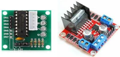
Fig.10 ULN 2003 BoardFig.11 L298N Motor Driver
