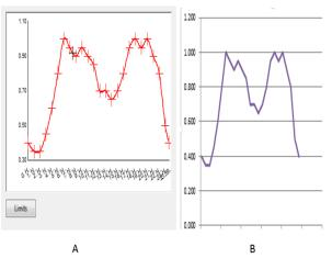
Figure 4 – Residential load profile representation in A) DIgSILENT B) MS EXCEL – Data from [5-6]
