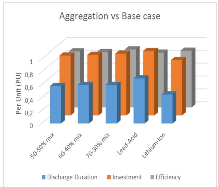
Fig. 9. Aggregated performance of battery options
