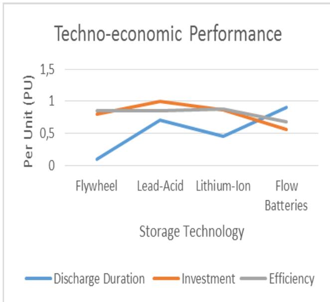
Fig. 8. Combined performance of battery options
