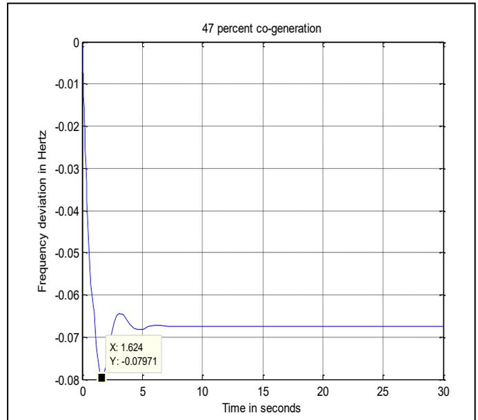
Fig. 4. Frequency behavior with 47% co-generation
