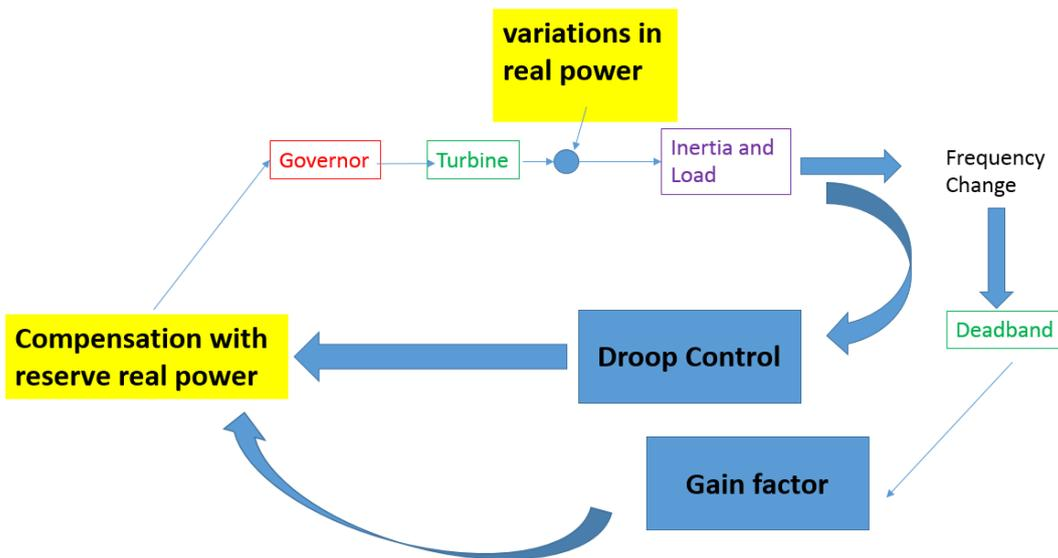
Fig. 1. Primary frequency control conventional technique – Conventional & Modified ([17])
