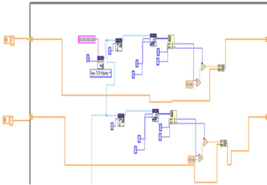
Fig. 4. Buffer for Reactive Power Readings
