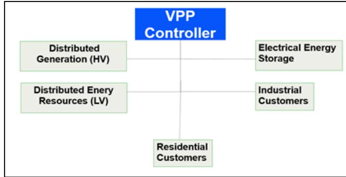
Fig. 1. Architecture of Virtual Power Plant
