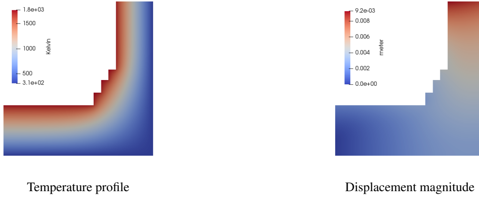
Figure 6.14: Temperature and displacement profiles
