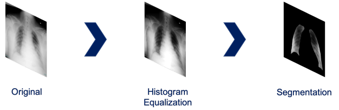
Fig. 1: CXR pre-processing steps proposed.
