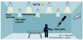
Figure 1. Example of VLC-based IoT scenario for home automation.
