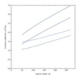
**Figure 1**. Results of recalculation by Mathematica 12.0 of the translational friction coefficients for "dumbbell" (upper curves) and "lollipop" (lower curves) reference assemblies, for comparison to Figure 2 of the original article. Each assembly was calculated using the presented approach (solid line) and the standard approach (dashed line). The original figure also depicted corresponding "exact" data points for reference, as calculated by other authors.
