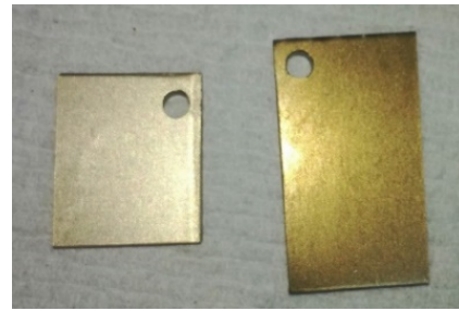
Figure 1: Optical image of hexagonal silver NbN film (left) and cubic gold NbN film (right).
