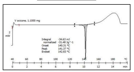
Fig. 1: DSC Thermogram of pure Oxiconazole nitrate.
