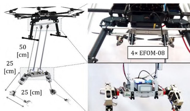
FIGURE 9. Detailed view of the integration of the compliant dual arm in the aerial platform in pendulum configuration.
