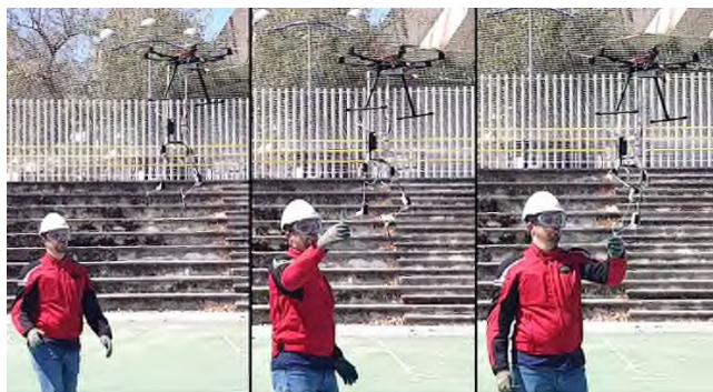
FIGURE 4. Aerial tool delivery with close human interaction using a dual arm aerial manipulator in long reach configuration.
