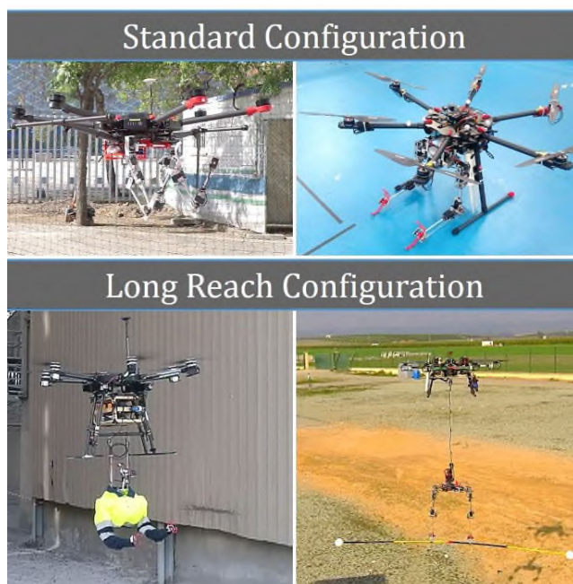
FIGURE 1. Compliant dual arm aerial manipulators in standard (up) and long reach/passive pendulum (down) configurations.
