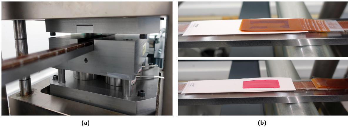
Figure 3.4: (a) Specimen 1 (cable HT15OC0190) in the pressing tool and (b) 1-mm-thick polyimide foil stack intermediate layer (top) with pressure-sensitive films (bottom) after applying a nominal stress of 175 MPa.
