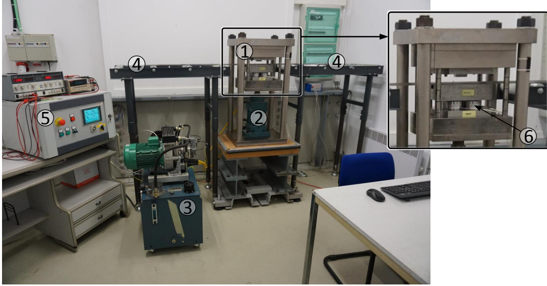
Figure 3.1: Setup for applying transverse compressive stress on the cable and wire specimens. 1. Pressing insert, 2. Hydraulic jack, 3. Hydraulic circuit, 4. Supports with support bar, 5. Control unit, 6. Load cells.
