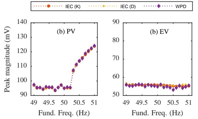
Fig. 5. Magnitude of the 16 kHz peak of the PV inverter (a) and of the 20 kHz peak of the EV charging system (b) at varying power frequency, assessed with different measurement methods.
