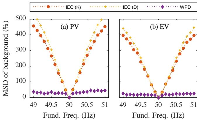
Fig. 6. Comparison of the variations of the background at varying power frequency, with different measurement methods. The PV inverter is shown in (a) and the EV charger in (b).
