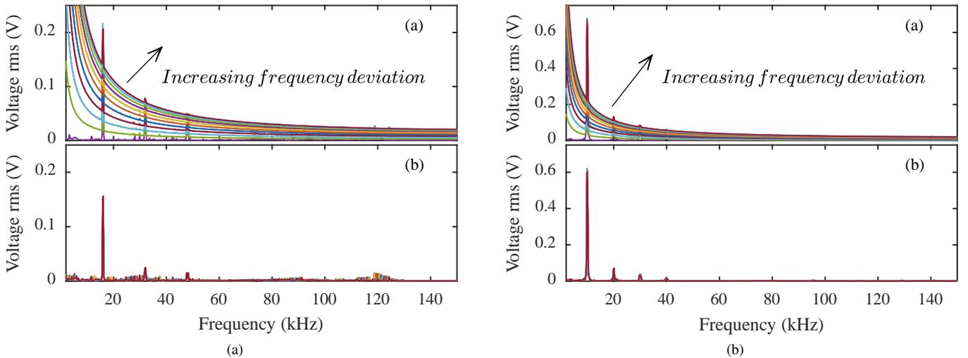
Fig. 3. Comparison of voltage spectra measured with IEC method (top) and WPD method (bottom) at varying power frequency. A PV inverter is shown in (a), while a and a EV charger is shown in (b).
