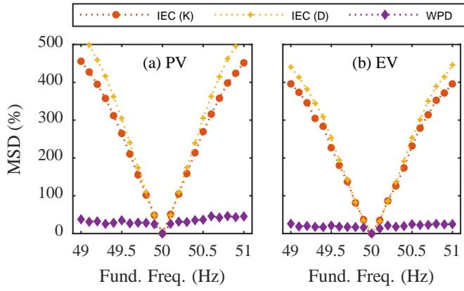
Fig. 4. Variations in the results of the different measurement methods at varying power frequency. The PV inverter is shown in (a) and the EV charger in (b).
