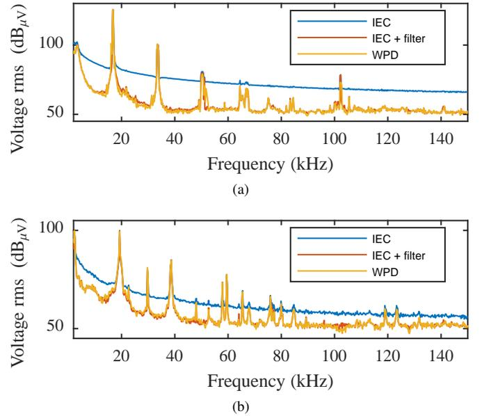
Fig. 2. Voltage of PV inverter (a) and an EV charger (b) measured on the grid and analyzed with the proposed method and the IEC method (with a previous filtering stage according to [9] and without filtering).
