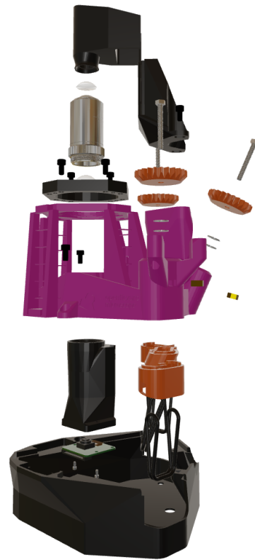
Fig. 1. Exploded view of the OpenFlexure Microscope.
