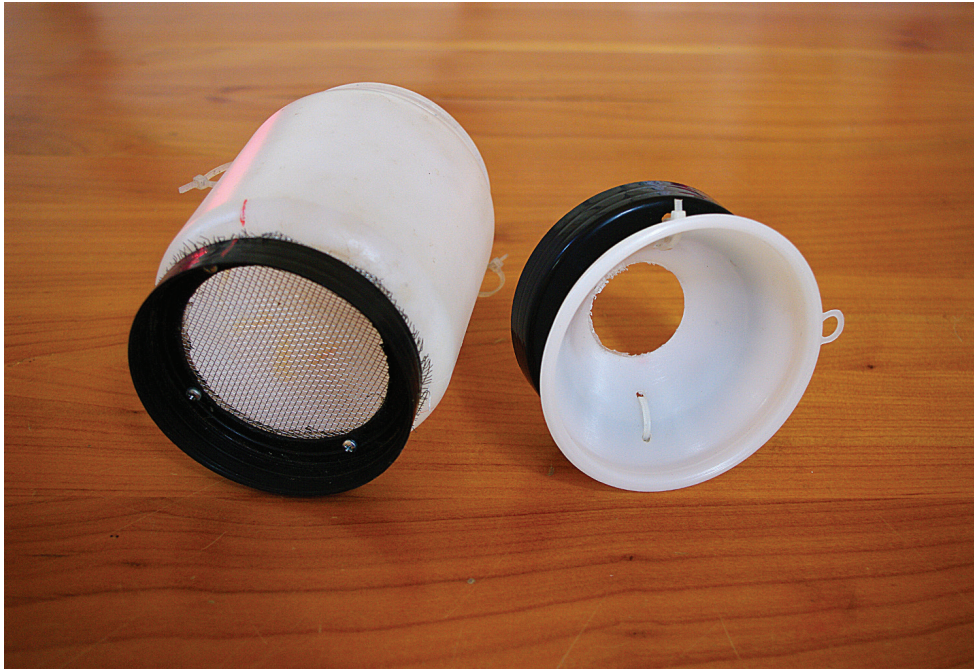
Figure 3. The upper jar of the baited trap modified with a wire insect net and a modified lid in which a plastic funnel has been inserted to collect insects falling into the trap (Photo by M. Bardiani).
