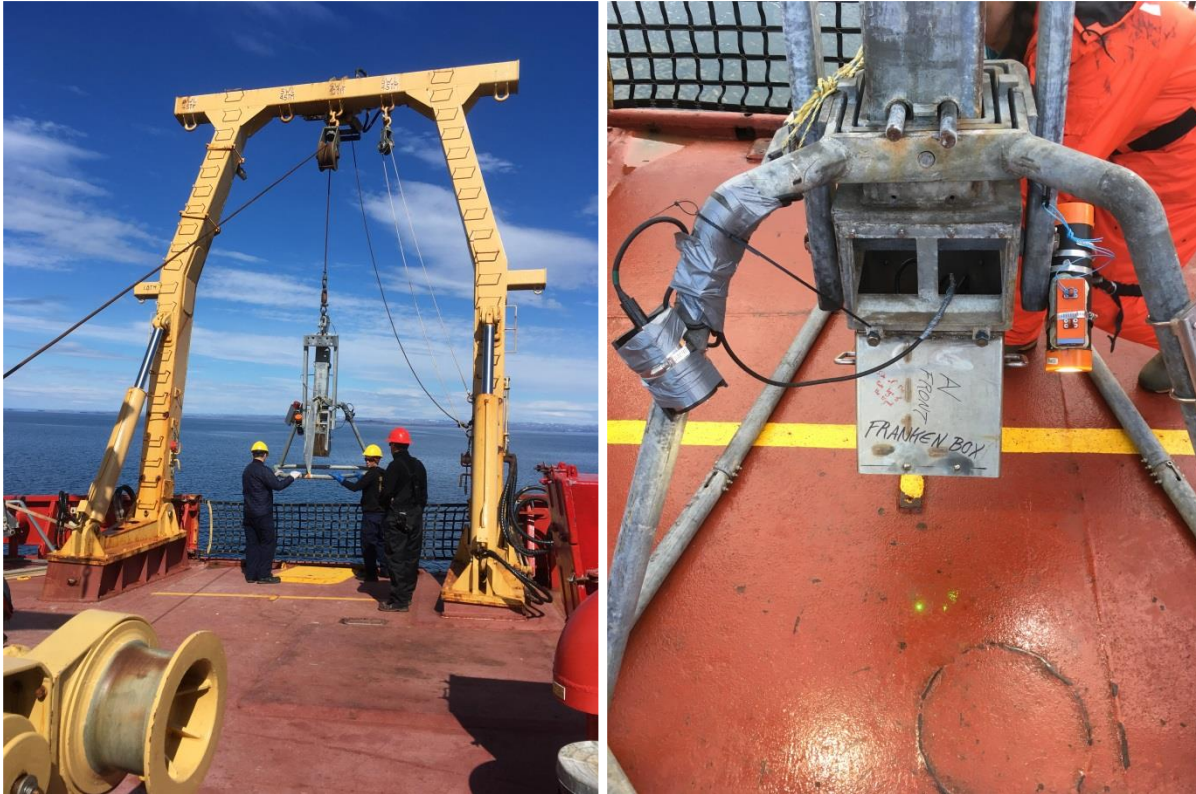
Figure 3: The drop camera system attached to a modified box core frame utilized in Leg 1b of the 2019 Amundsen Expedition.
