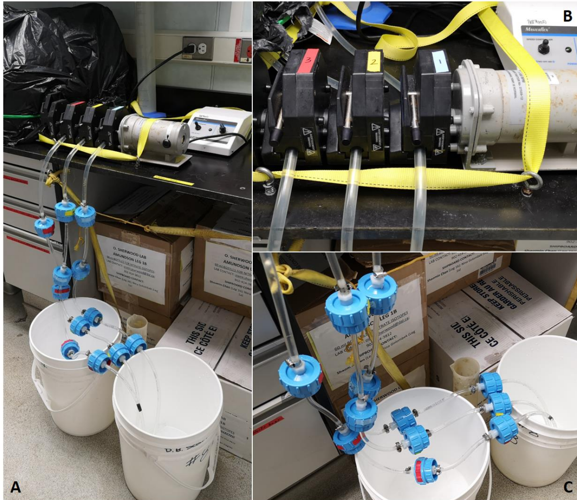
Figure 2: Overview of the filtration system (A). The setup of the pump for filtering 3 samples at the same time (B) and the 4 different-size filters in the filter holders for each sample with 180 \mu\text{m} filter at the near-pump end and 0.2 \mu\text{m} filter at the near-bucket end (C). Samples were covered by a dark bag during the filtration.
