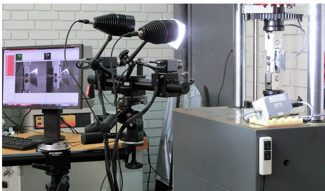
Figure 2 Experimental set-up for fatigue testing
