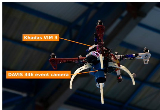
Fig. 1: Aerial robot based on DJI Flamewheel F450 equipped with a DAVIS 346 event camera and a low-cost Khadas VIM3 used for on-board computation.
