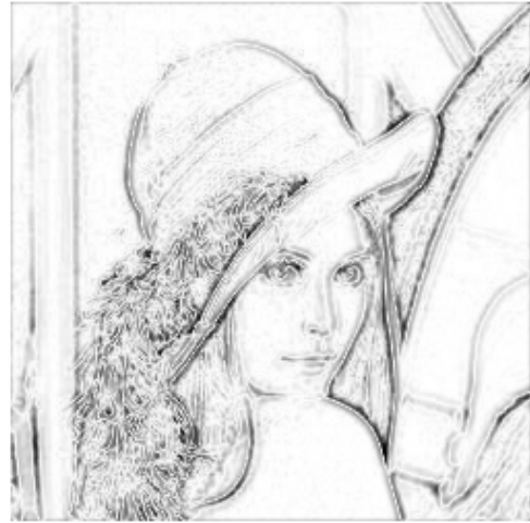
Figure 9: Edge intensity map of the Lena test image computed according to the proposed method, using a blurring by 5 x 5 neighborhood averaging.
