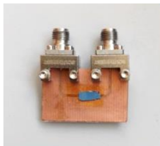
Figure 1: Image of the home-made U-shaped GCPW, where a Co/ \text{Sb}_2\text{Te}_3 sample is glued across the signal line. A small piece of mylar foil is positioned between the sample and the board in order to avoid electrical shortening of the line.
