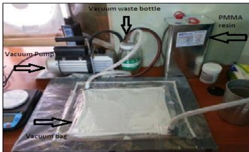
Figure (2): Vacuum bagging technique.
