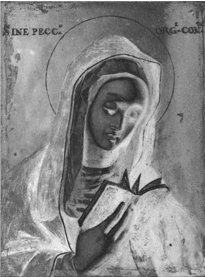
Figure 6 - Painting A: result of combining the UV and the induced-fluorescence images. Punctual discontinuities in the pictorial layer are highlighted.
