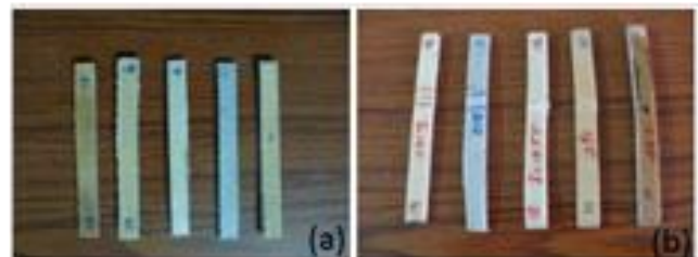
Fig. 4 Experimental Fatigue Specimen, (a) Before and (b) After Test.
