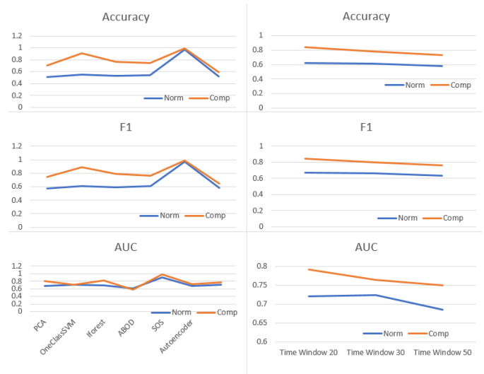
Fig. 5: The overall performance of the machine learning and deep learning methods with and without the proposed complex feature representation and the affect of the size of the sliding time window.
