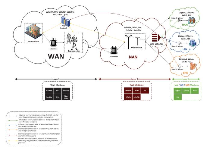
FIGURE 3. The SG architecture in terms of communication.
