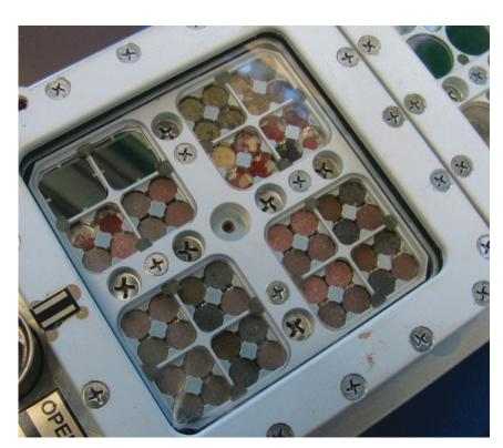
**FIG. 1.** Mars analog pellets integrated in the EXPOSE-R2 hardware.
