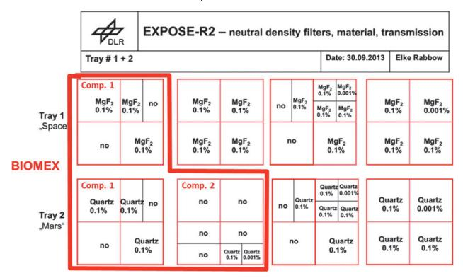
FIG. 5. The distribution of neutral density filters and the values of transmission depending on the used material.
