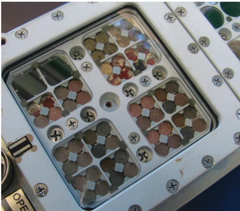
FIG. 1. Mars analog pellets integrated in the EXPOSE-R2 hardware.
