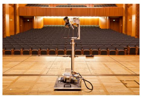
Figure 15 Canon EOS 5D camera mounted on the VariSphear system
