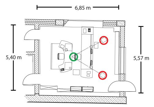
*Figure 2 Sketch of the CR1 (green circle = listener position (receiver) / red circle = sound sources)*
