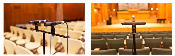
Figure 14 Example for a stereophonic configuration (left picture: Small AB with Schoeps MK2, right picture: ORTF with Schoeps MK4)
