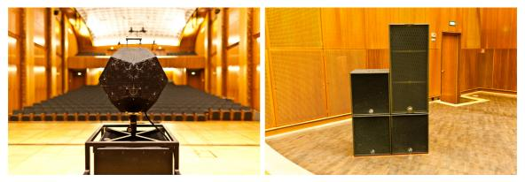
Figure 18 Omnidirectional source: The high power wideband dodecahedron "Sonic Ball" (left picture) and the horn loaded PA rig from AD-Systems (right picture)
