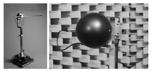
*Figure 12* VariSphear scanning array system in an open sphere configuration (left picture) and with the rigid sphere extension and the Earthworks M30 microphone (right picture).
