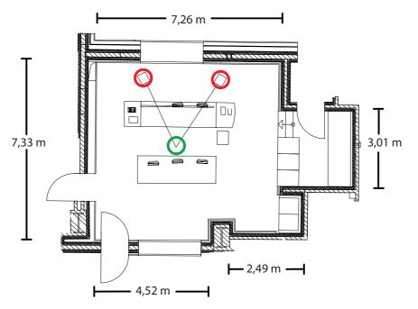
*Figure 4 Sketch of the CR7 (green circle = listener position (receiver) / red circle = sound sources)*
