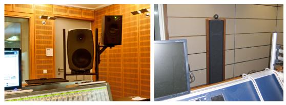
*Figure 17* The used main monitor systems: Genelec 8260A in CR1 (left picture) and B&W 803D in CR7 (right picture)
