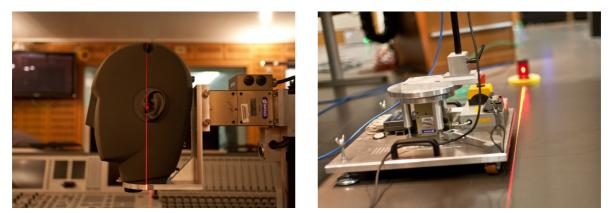
*Figure 11* Examples for a very accurately conducted laser based calibration. (left picture: Neumann KU100 in CR1; right picture: VariSphear ground plane in CR7)
