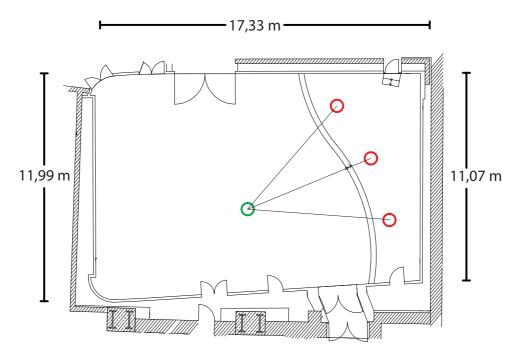
*Figure 6 Sketch of the SBS (green circle = listener position (receiver) / red circle = sound sources)*
