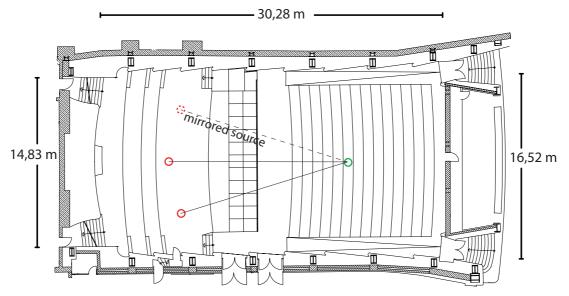
Figure 9 Sketch of the LBS (green circle = listener position (receiver) / red circle = sound sources)
