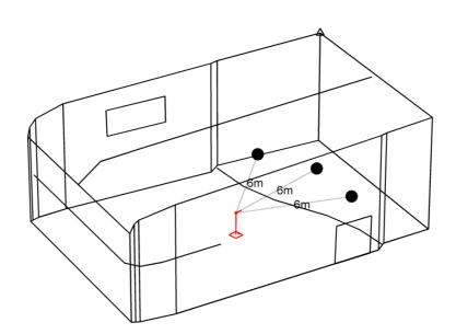
Figure 16 Exemplary CAD model of the small broadcast studio. Additionally the measures like lengths, surfaces or the room volume could be included, but for the ease of exposition the presented model is kept simple. The three bubbles on stage demark the sources and the red structure in the center depicts the array.
