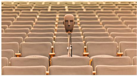
Figure 13 KU100 mounted on the VariSphear system (ROTM) in the large broadcast studio
