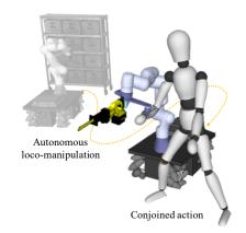
Fig. 1: The proposed control framework aims to incorporate the advantages of cobots and supernumerary limbs into a unified collaborative framework, to cover a large range of industrial task requirements.
