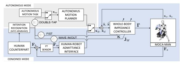
Fig. 4: The overall control architecture of the presented collaborative framework.
