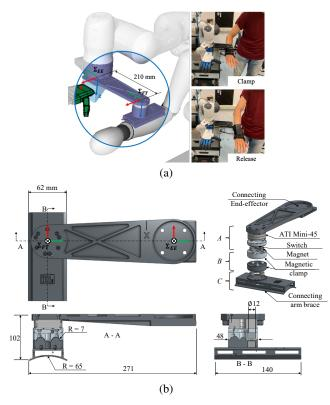
Fig. 3: The components of the developed human-MOCA admittance interface: *A*-robot mounting part, *B*-magnetic clamp part and *C*-wearable part. The admittance interface can be attached/detached through a magnetic clamp.
