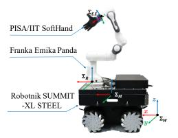
Fig. 2: Illustration of the MObile Collaborative robotic Assistant (MOCA) and the reference frames: world frame  $\Sigma_W$ , mobile platform base frame  $\Sigma_M$ , robotic manipulator base frame  $\Sigma R$ , and endeffector (SoftHand) frame  $\Sigma_{EE}$ .
