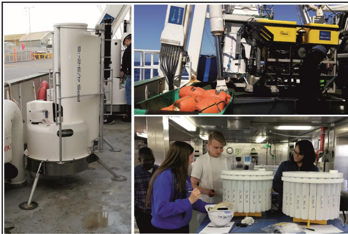
Fig. 5 left: lander; top right: lander mounted on the ROV and; bottom right: lander internal sampling bottles.
