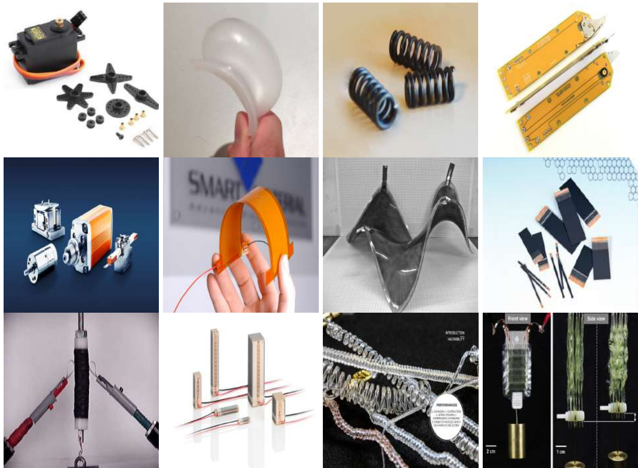
Fig. 1. From left to right and up to down: 1) Commercial available traditional servo motor; 2) Pneumatic actuator out of "Ecoflex"; 3) SMA springs; 4) SMA linear actuator; 5) Commercial piezo motors; 6) MFC out of NASA; 7) PEA actuated sheet; 8) Commercial EAP plates; 9) Stacked PEA concept; 10) Commercial stacked PEA for low displacement, 11) Different configurations of TCP; 12) Peano-HASEL actuator.
