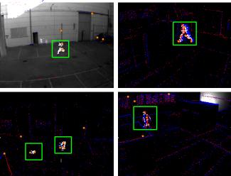
Fig. 3: Intruder monitoring during four experiments. From top-left: (i) daylight, (ii) night, (iii) multi-object, and (iv) illumination changes. Cluster events and feature tracks are represented by white and orange pixels respectively.
