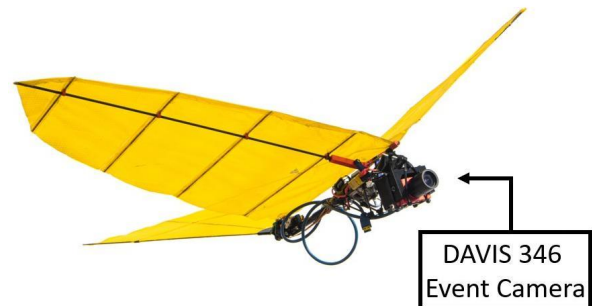
Fig. 1: GRIFFIN ornithopter prototype developed by the University of Seville equipped with an onboard DAVIS 346 event camera.
