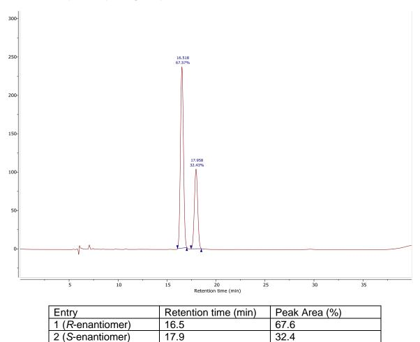
5.1.11 Sav:1 (1 mol%) using 5 equivalent of acetone and 25% acetonitrile
