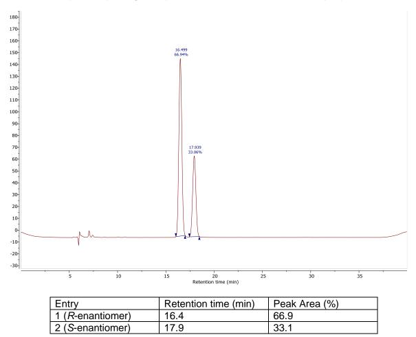
5.1.13 Sav:1 (1 mol%) using 50 equivalent of acetone and 25% iso-propanol
