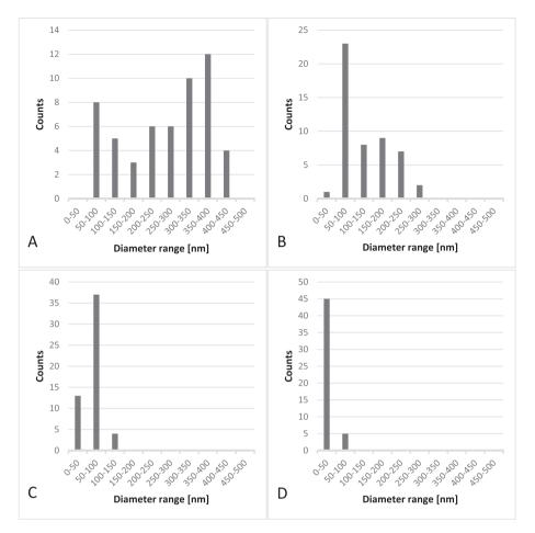
Fig. 3. Histograms of diameters for green composites (A, B) and calcined fibers (C, D) produced from PVA/Th(NO<sub>3</sub>)<sub>4</sub> (A, C) and PVP/Th(acac)<sub>4</sub> (B, D).
