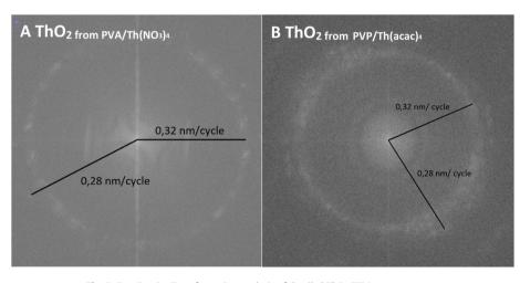
Fig. 6. Fast Fourier Transformation analysis of detailed ThO<sub>2</sub> TEM measurements.
