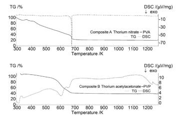
Fig. 1. TGA/DSC measurements of green composites from solutions A (top) and B (bottom).
