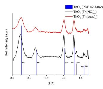
Fig. 4. PXRD measurements of calcined samples. Used lamp Co K $\alpha$  1.79030 Å. X axis: d [Å], Y axis: relative intensity.
