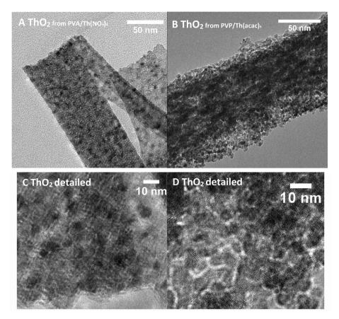
Fig. 5. The TEM analysis of calcined products (A, B) with details of nanocrystalline structure (C, D) produced from PVA/Th(NO<sub>3</sub>)<sub>4</sub> (A, C) and PVP/Th(acac)<sub>4</sub> (B, D).
