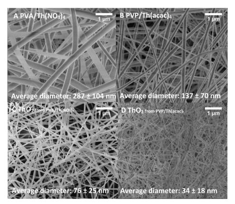
Fig. 2. SEM micrographs of green composites (A, B) and calcined fibers (C, D) produced from PVA/Th(NO<sub>3</sub>)<sub>4</sub> (A, C) and PVP/Th(acac)<sub>4</sub> (B, D).
