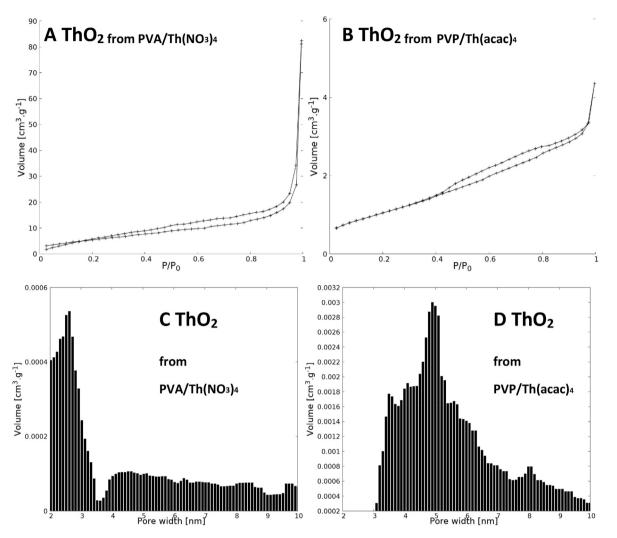
Fig. 7. Adsorption/desorption isotherms and corresponding pore size distributions determined by the DFT method of ThO<sub>2</sub> nanofibers prepared from PVA/Th(NO<sub>3</sub>)<sub>4</sub> (A, C) and PVP/ Th(acac)<sub>4</sub> (B, D).
