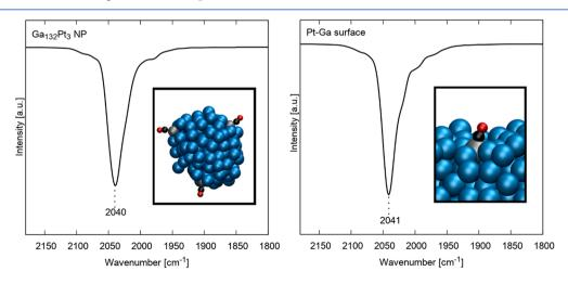
Figure 4. Vibrational spectra for the CO vibration on the Ga<sub>132</sub>Pt<sub>3</sub> NP (left) and the slab model (right) calculated from the velocity–velocity autocorrelation function of AIMD simulations. Ga, Pt, C, and O are depicted in blue, silver, black, and red, respectively.
