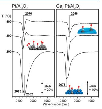
Figure 3. DRIFT spectra obtained during CO adsorption on two Pt-containing catalysts, namely,  $Pt/Al_2O_3$  and  $Ga_{37}Pt/Al_2O_3$ .
