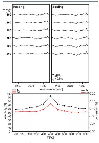
**Figure 5.** (top panel) Operando DRIFT spectra recorded on the  $Al_2O_3$  sample at selected temperatures. (bottom panel) Conversion of propane for the  $Al_2O_3$  sample.
