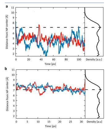
**Figure 2.** Distance from the NP center for two selected Pt atoms as a function of time as obtained in ab initio molecular dynamics (AIMD) simulations. The Pt atoms were initially located at the surface: (a) without adsorbed CO, (b) with adsorbed CO. The Ga density (a.u., arbitrary units) is plotted for comparison; the dashed line resembles the first maximum in the Ga density.
