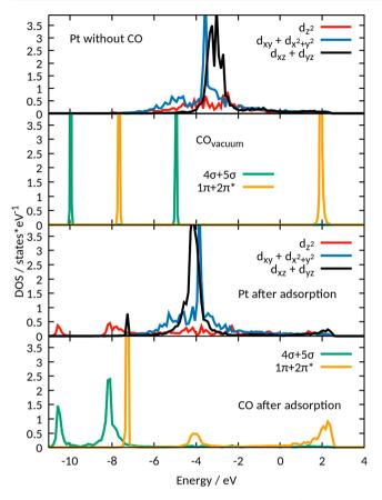
**Figure 9.** Orbital-resolved electronic density of states (DOS) on Pt model systems before and after adsorption of CO (see text for details).
