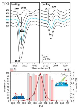
**Figure 8.** (top panel) Operando DRIFT spectra recorded on the  $Ga_{37}Pt_1/Al_2O_3$  SCALMS sample at selected temperatures. (bottom panel) Conversion of propane and selectivity toward propene for the  $Ga_{37}Pt_1/Al_2O_3$  SCALMS sample (lines are guides to the eye).
