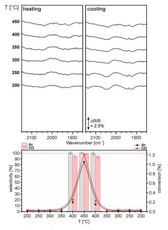
**Figure 6.** (top panel) Operando DRIFT spectra recorded on the Ga/ $Al_2O_3$  sample at selected temperatures. (bottom panel) Conversion of propane and selectivity toward propene for the Ga/ $Al_2O_3$  sample (lines are guides to the eye).
