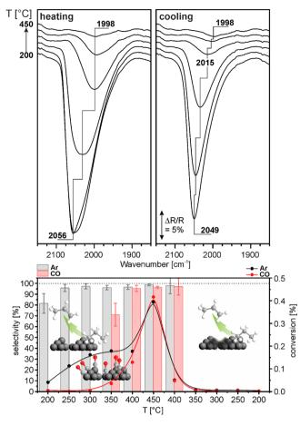
**Figure 7.** (top panel) Operando DRIFT spectra recorded on the Pt/ $Al_2O_3$  sample at selected temperatures. (bottom panel) Conversion of propane and selectivity toward propene for the Pt/ $Al_2O_3$  sample (lines are guides to the eye).
