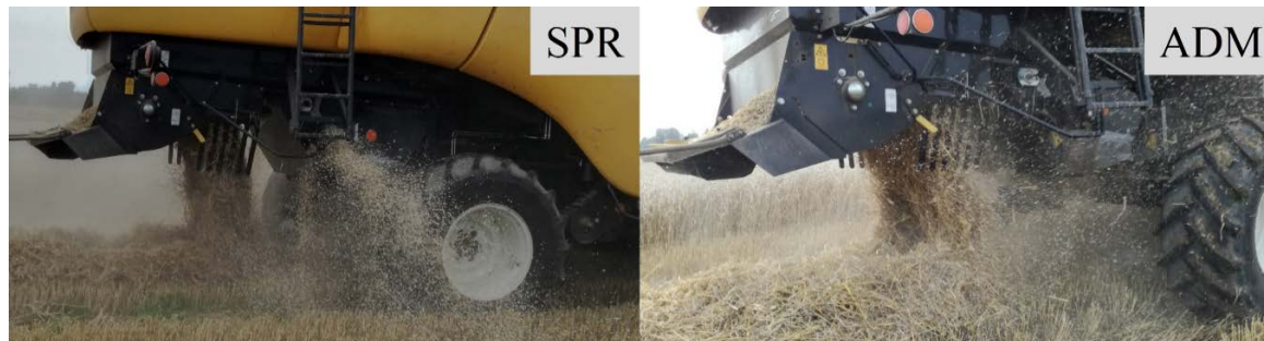
Figure 1. Chaff mixing strategies applied in the present study: the chaff was either spread (SPR, left panel) on the soil laterally to the straw swath by the combine harvester or it was admixed to the straw and released at the same time (ADM, right panel) (Source: CREA).
