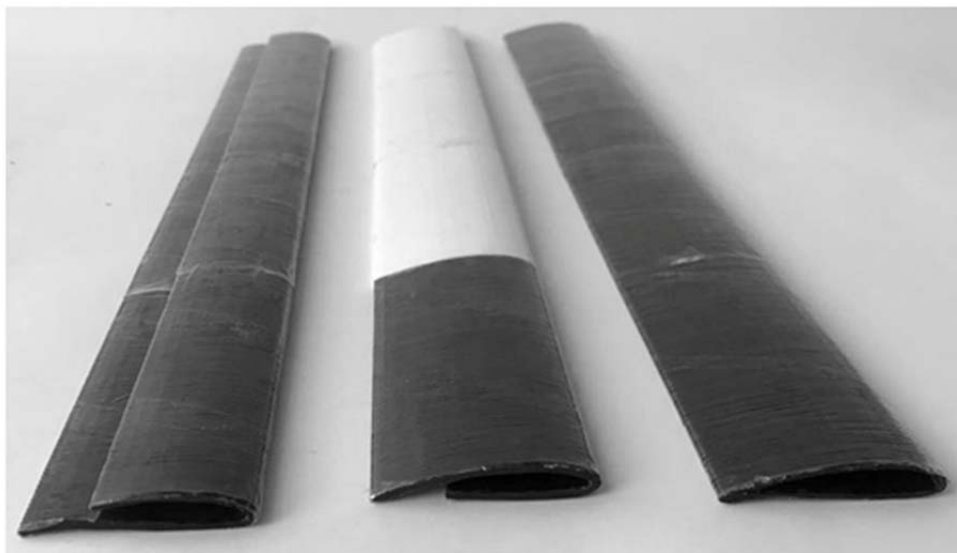
Figure 10. 3D printed opened and full blades, FX 63-137 airfoil.
