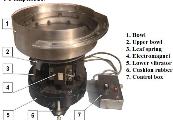
Fig. 1. Automatic vibratory bowl feeder
